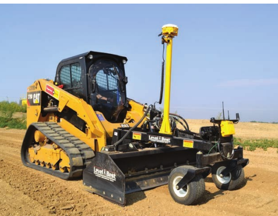
ATI Level Best PD Series Grading Box and Trimble GCS900 Grade Control System with Single GNSS
