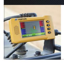
Configure the i-33 system with a single GNSS or dual GNSS antennas and install it on different machines that require elevation indication. Installation requires minimal welding on the machine, this makes the i-33 easy to switch between a dozer, scraper, or motor grader.
