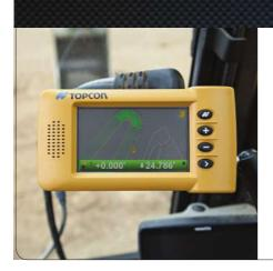
The Topcon X-33 system consists of two GNSS antennas, four TS-i3 tilt sensors, the MC-i3 GNSS receiver and the GX-30 color, touch screen control box. The GX-30 allows the operator to "see" the exact position of the machine on site and the bucket position at all times. When detailed information is required you can select to visualize plan, profile or sectional view and use the dual grade indicators for elevation control.
